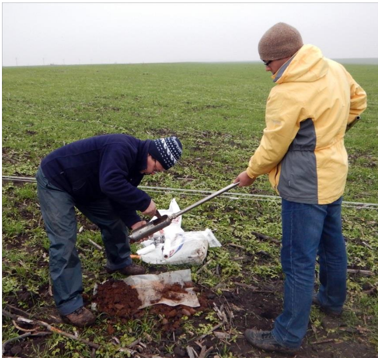
Figure 8.1. Soil probe used for coring.
